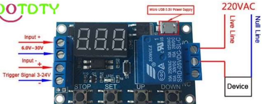
Low Voltage Control High Voltage Connection Picture
